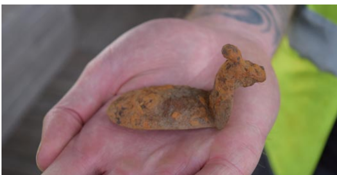
A mechanism of Musket furniture: A frizzen (BA17HOU_1742) (a piece of steel used to produce a spark when struck by the musket flint) considerably worn due to use in combat
