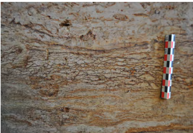
Figure 12 - Iron panning, caused by compaction at the base of the hollow.
